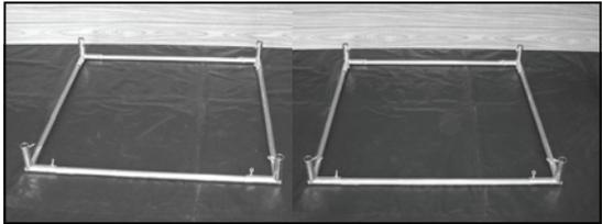
2. Insert swaged pipes into each corner of one square and the remaining unswaged pipes into the four corners of the other square
